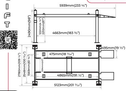
8500 LBS **CAPACITY** 110 volts. **20** amp electrical circuit
